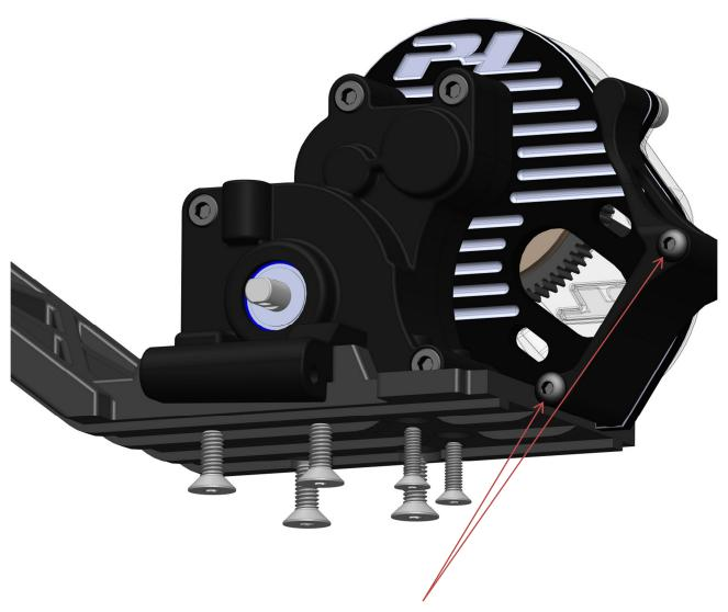
\*Slash Requires removal of these screws before installation\*
