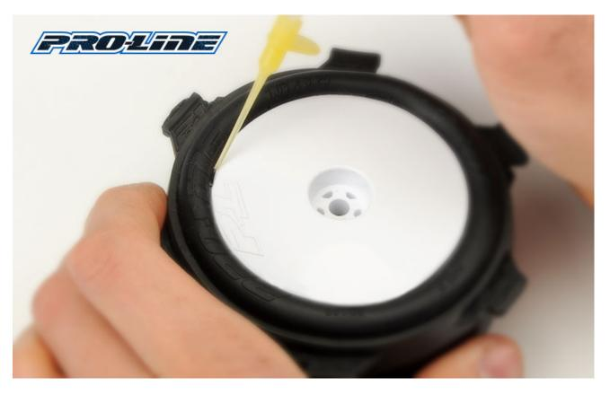
Finally run a thin layer of glue around the outer edge of the bead. Set the wheel aside and allow plenty of drying time before moving to the other side.
