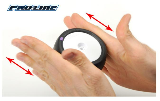
With the foam inserted and the tires in place on the wheel, roll the tire back and forth between your hands in to check the foam and tire bead are properly seated onto the wheel.
