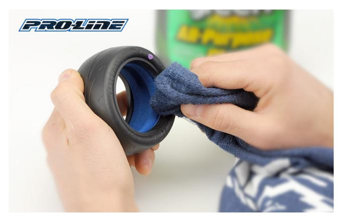
Residual lubricants from the manufacturing process need to be removed from the gluing surfaces with a lint free towel and an all-purpose cleaner that will not leave behind any additional residue. Simple Green®, Windex®, and isopropyl alcohol are some favorites.
